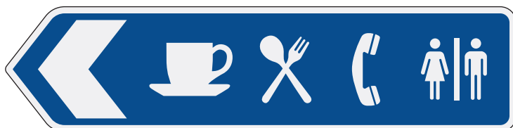
Figure 16.2 – Examples of symbols used in a MOTSAM motorist service sign
