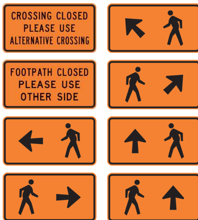
Figure 18.1 – Examples of temporary pedestrian warning signage
