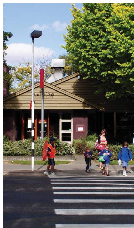
Photo 17.4 – Pedestrian crossing floodlit from lantern on black and white pole, in advance of crossing, Christchurch (Photo: Tim Hughes)
